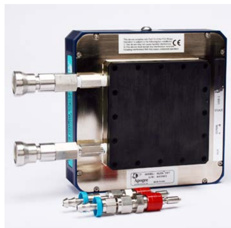
Alta camera adapted for liquid circulation with quick disconnects
